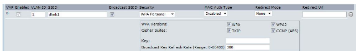
Figure 25 - Modify Virtual Access Point Settings (WPA Personal)
